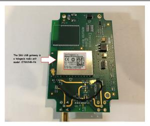
**Technical Background** - The IGS radio unit is a *Telegeses* ETRX2HR-PA Zigbee WIFI radio unit with an Ember EM250 processor. It has a 128k of program flash space and runs with the Ember ZNet5.0.1 stack. There is a wired bootloader on the USB serial port which conforms to the EBL (ember boot loader) format. (Software is developed in the C language using the xIDE compiler which creates "EBL" firmware files.
