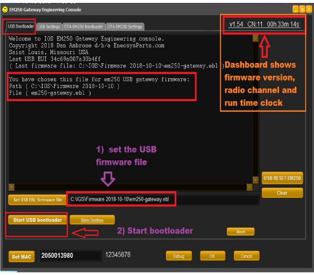
4) Click USB EM250 Bootloader. An Xmodem transfer box should appear and run a flash update that takes about 30 seconds.
